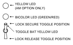
powered/unpowered status of the lock although this does not utilize the full capabilities of the panel.
